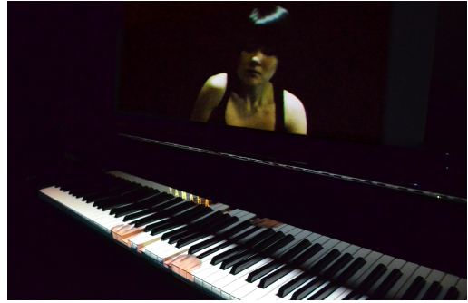
Figure 1: Photo of our interface. The hands and body of a projected virtual pianist are synchronized with moving keys of a player piano.
